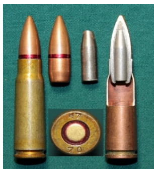
7,62-mm (PS) 1943 yil namunadagi patron patron po‘lat o‘zakli o‘qi bilan
