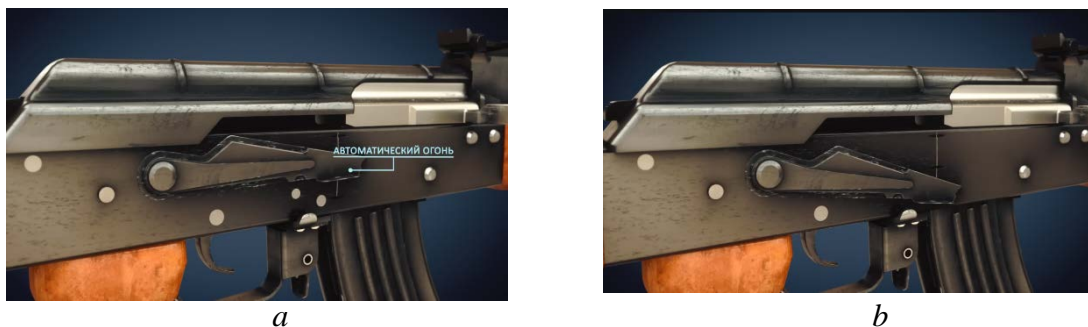
87-rasm. O‘tkazgichni zarur o‘q otish turiga qo‘yish: a – avtomatik tarzda o‘q otish uchun; b – bittalab o‘q otish uchun
