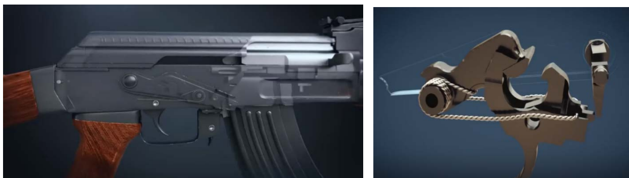
66-rasm. O'q otish o'tkazgichi (OD) xolatida
