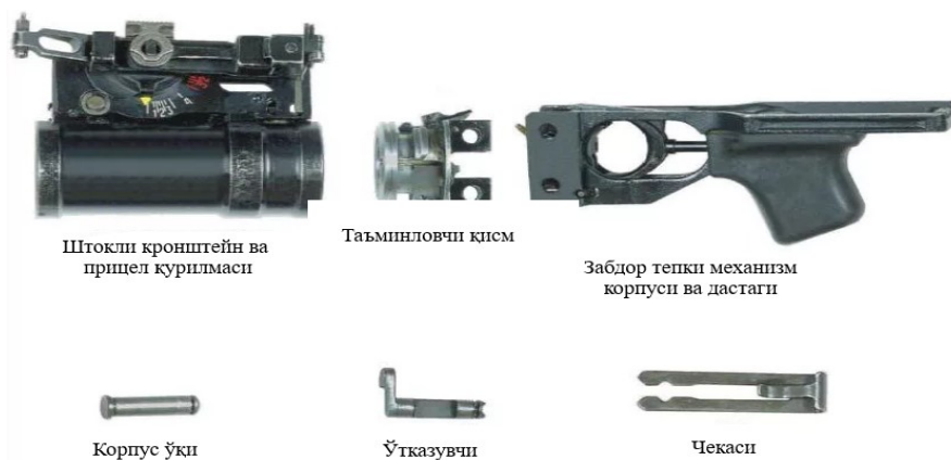
22-rasm. GP-25stvolosti granatomyotining asosiy qismlari
