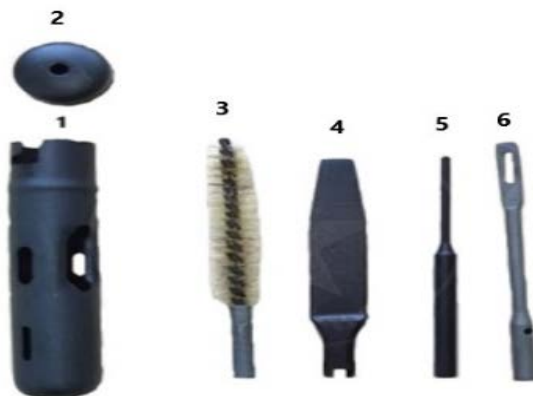
5-rasm. Penal anjomlari: 1 – Penal; 2 – Penal qopqog'i; 3 – artkich-cho'tka; 4 – otvyortka; 5 – chiqargich; 6 – tozalagich.
