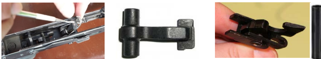
81-rasm. Tepkini stvol qutisidan ajratish hamda trubali o'qni ajratish
