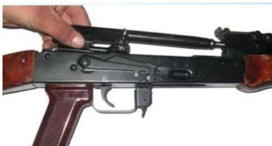
73-rasm. Zatvor ramasini zatvor bilan birgalikda ajratish
