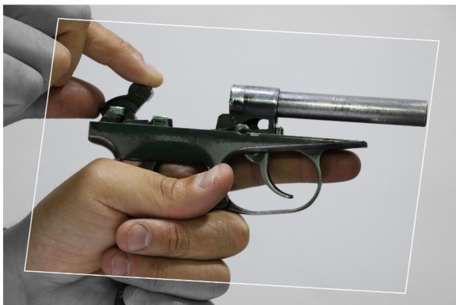
24-rasm. Tepkini ramkaga o‘rnatish.
