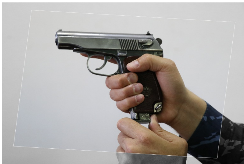
3-rasm. Magazinni dasta asosidan chiqarib olish
