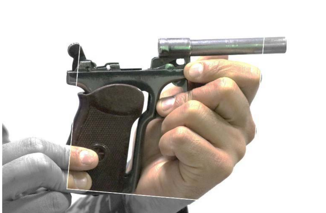
27-rasm. Zatvor ushlagich va sheptaloni ramkaga o‘rnatish.
