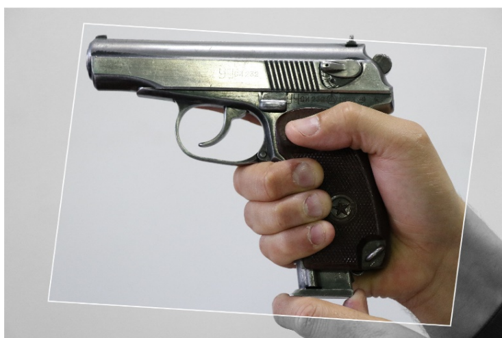
10-rasm. Magazinni dasta asosiga o'rnatish.
