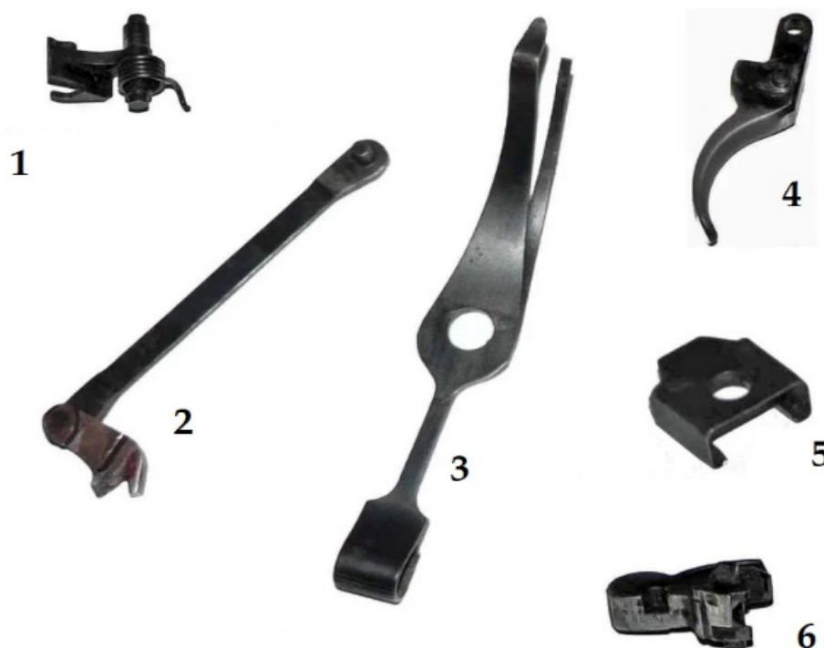
34-rasm. Zarbdor tepki mexanizmi: 1 – prujinali sheptalo; 2 – tepki tyagasi vzvod richagi bilan; 3 – jangovar prujina; 4 – tepki ilgagi; 5 – jangovar prujina surgichi; 6 – tepki.
