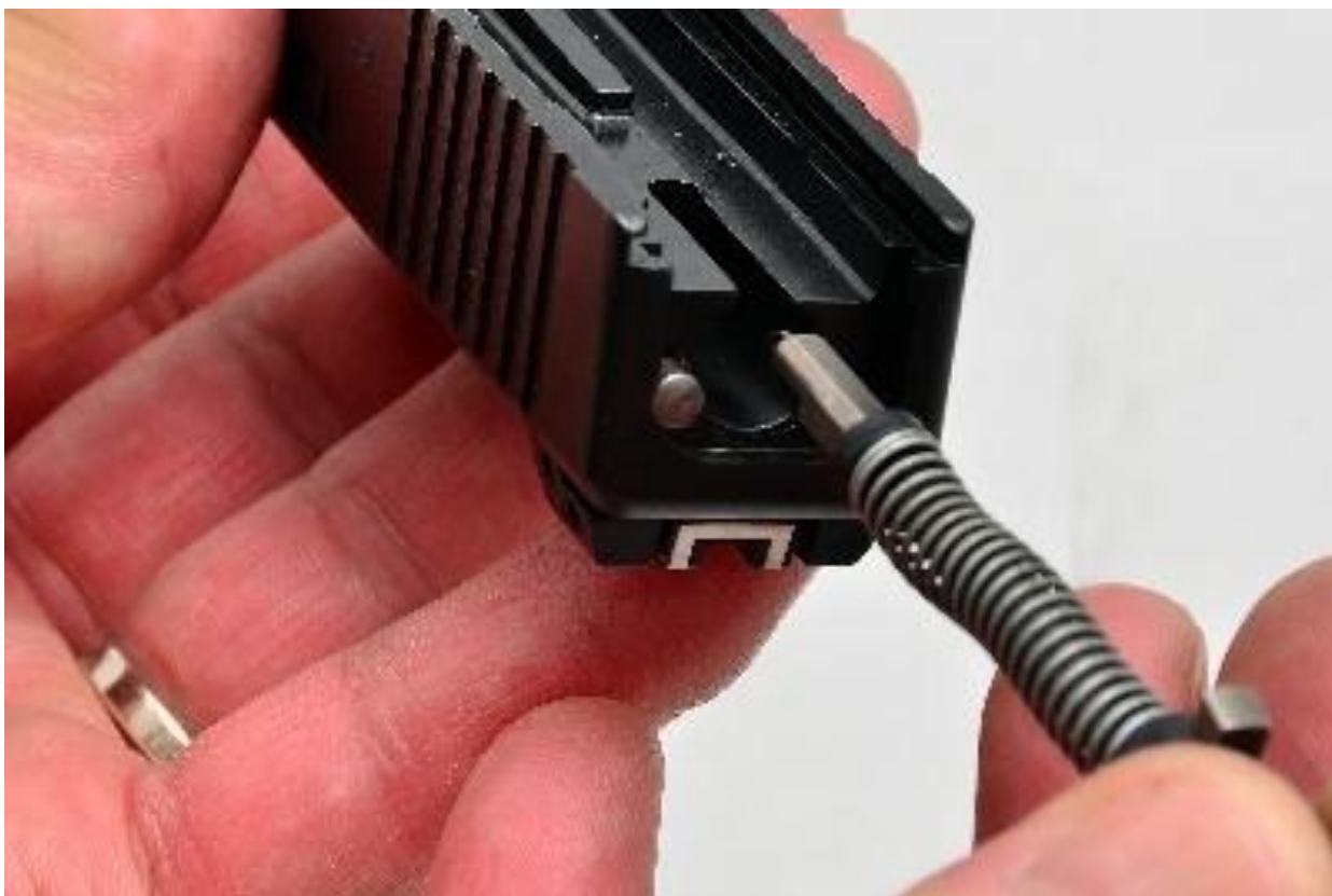
23-rasm. Jangovar prujinani chiqarib olish.
