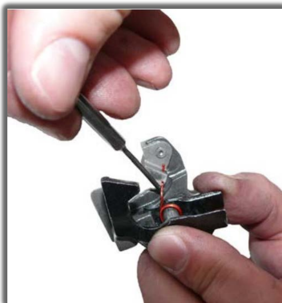
99-rasm. Sekinlatgich prujinasini o'rnatish
