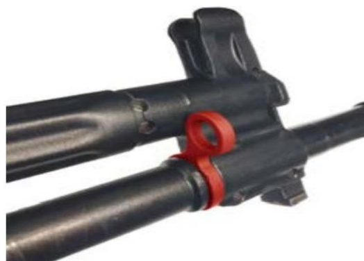
43-rasm. 6G15 stvolosti granatomyotini o'rnatish uchun antabkaning zaruriy holati
