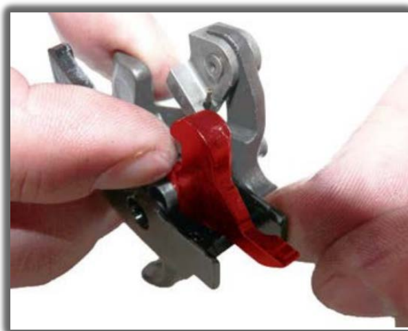
97-rasm. Yakkalab otish sheptalosini o'rnatish
