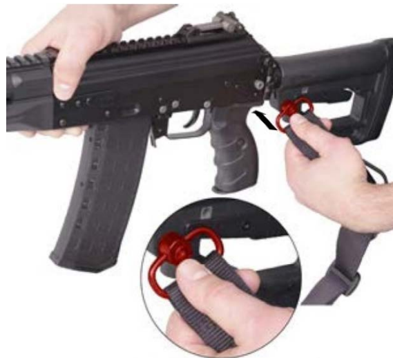
50-rasm. Tasma antabkasini qo‘ndiq to‘plami korpusining vtulkasiga kiritish
