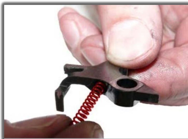
98-rasm. To'xtatish sheptalosi prujinasini o'rnatish
