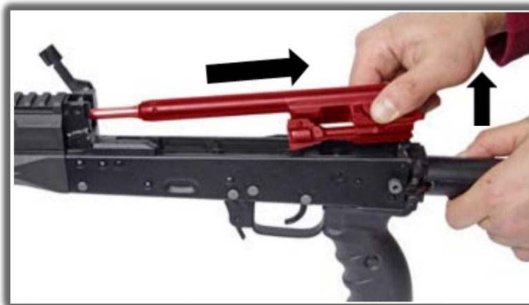
64-rasm. Zatvor ramasini zatvor bilan birga ajratish.
