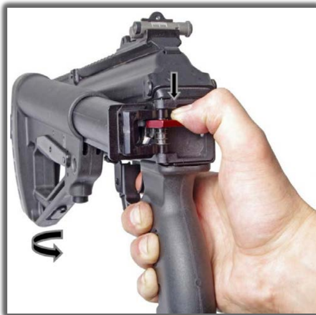
30-rasm. Qo'ndiq safar holatida jangovar holatga keltirish
