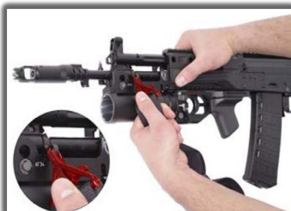
55-rasm. 6G34 stvolosti granatomyoti o‘rnatilgan avtomat antabkasiga tasma karabinini kiritish
