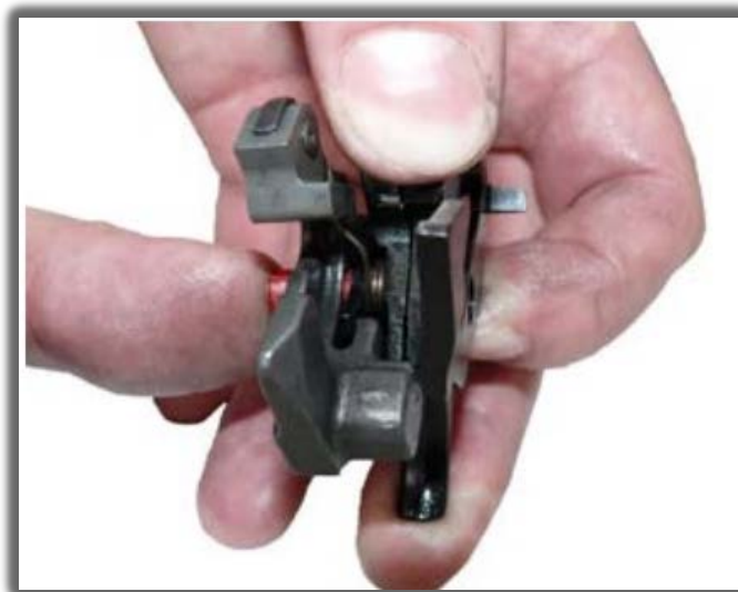
100-rasm. To'xtatish sheptalosining o'rnatish
