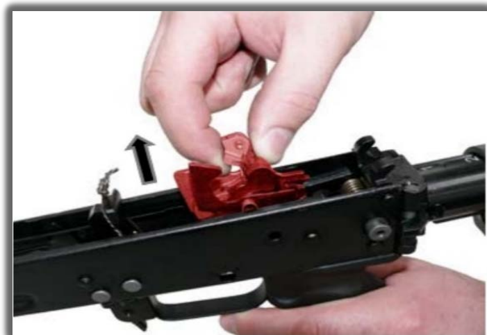
86-rasm. Tepki mexanizmi tugunini ajratish
