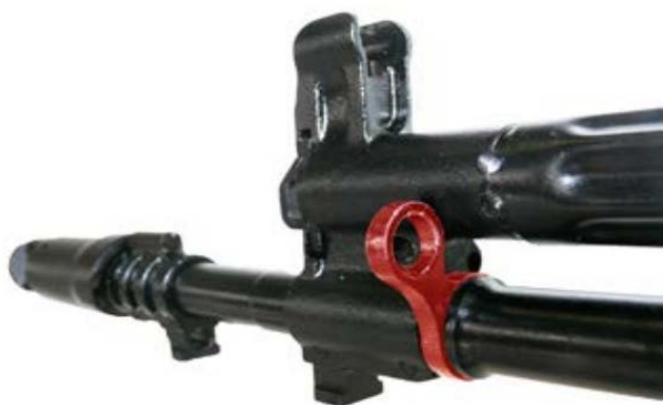
42-rasm. 6G34 stvolosti granatomyotini o'rnatish uchun antabkaning zaruriy holati
