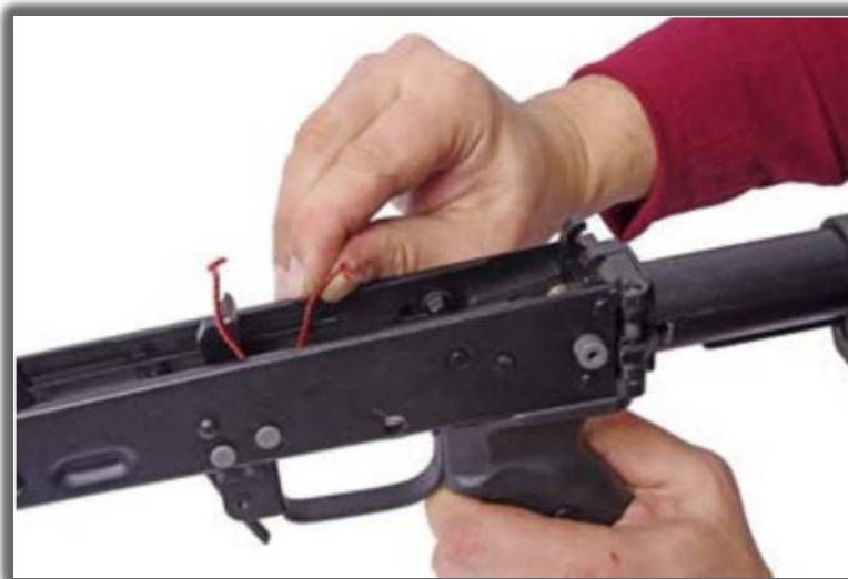
83-rasm. Jangovar prujinaning o'ng uchini tepking jangovar vzvodi orqasiga keltirish
