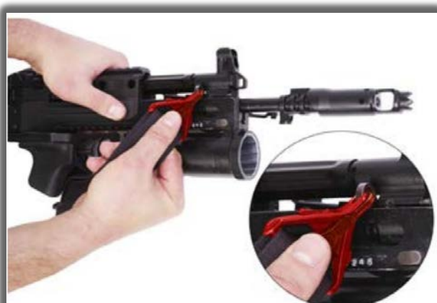
56-rasm. 6G15 stvolosti granatomyoti o‘rnatilgan avtomat antabkasiga tasma karabinini kiritish
