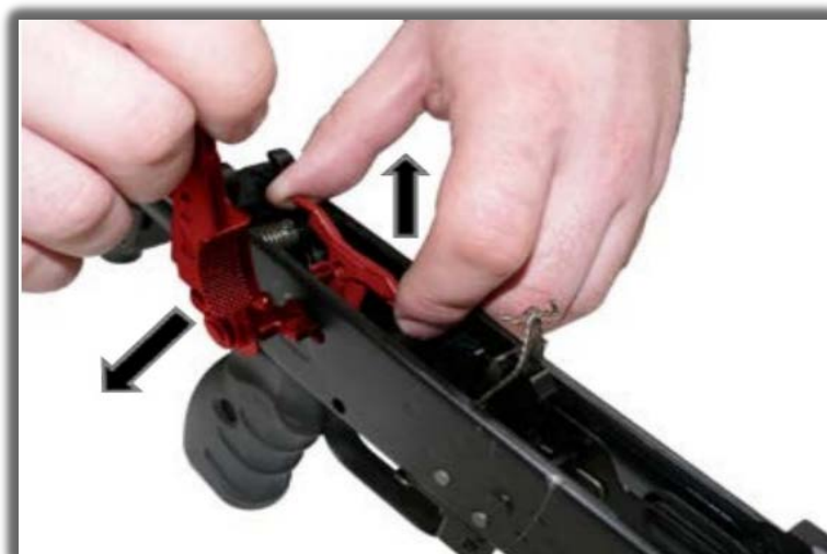
85-rasm. O'tkazgichni ajratish va to'xtatish mexanizmini yechib olish
