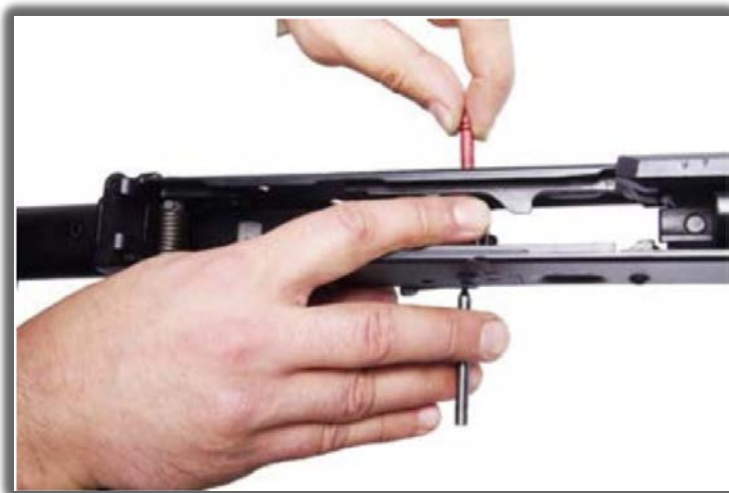
91-rasm. Avtospusk o'qini o'rnatish.
