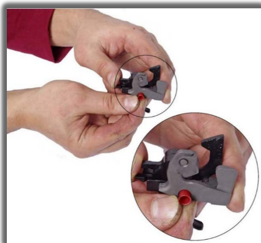
87-rasm. Vtulkani chiqarib olish
